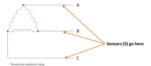
Note: The sensor position is the same for Delta, High-Leg Delta or Corner Grounded Delta systems.
