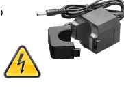
**3.2** Connect sensors, Ethernet cable (if using) and power adapter to the Eyedro module.
